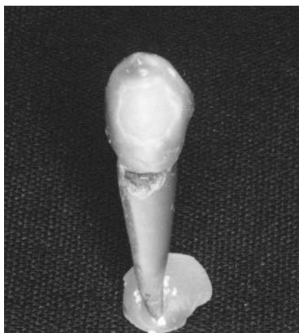
Figure 1. Waxed out crown with exposed labial surface after 72-hour exposure to test solution.
