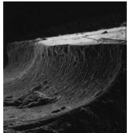
Figure 5. Regular Coke on a surface which had been etched and sealed with a light-cured sealant prior to submersion. 300x magnification.
